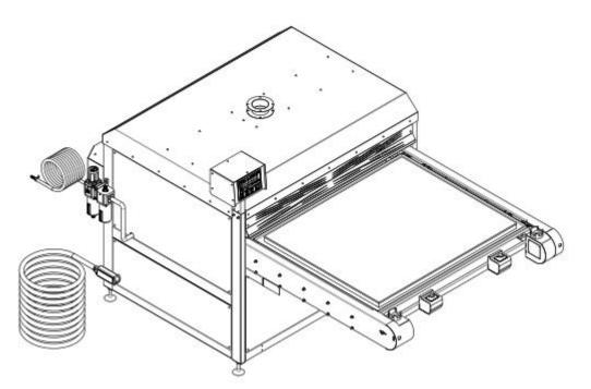
8. The machine finished assemble. Make sure the good ventilation and then to do the testing.
