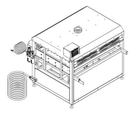
2. Check and make sure there is no any parts of the machine is missing or damaged during the shipping process. Demount the left and right panel, as shown above.
