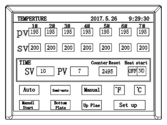
2)Press 1 # corresponding to set the SV position, enter the # 1 to the heating zone temperature setting, press ENT to save and then exit, CLR to clear the setting, ESC to reset; The same way for setting 2 to 6 #; Press switch in degrees Celsius or degrees ; After the setting, press the heat start to open the heating switch, the machine wil enter into the heating mode.
