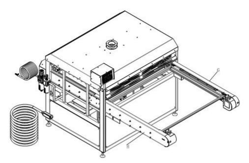
5. Install the left front plate of slide track H and right front plate of slid track G, lock the screw well.
