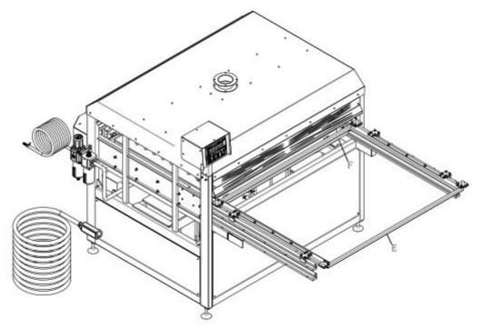
4. Fixed the slide tracks on the machine, Install the sliding frame E,F to the slide tracks. As shown above.
