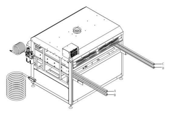
3. Demount Upper, Left and Right panel, then install the slide tracks. Fix the A,B,C,D slide tracks to the hole of the machine frame, as shown above(Fix the screw not to lock well)
