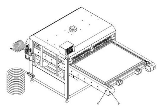
7. To adjust P points, This is the adjusting screw bolt of tension synchronous belts. Lock the screw bolt after tension the synchronous belts on O points.
