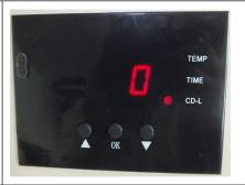
Press button after time setting; the display shows the temperature starts to rise. "CD-L" shows the time counting down during your transfer.
