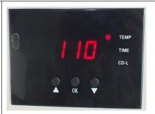
Press button, the temp light is on. Select with arrows the temperature according to different transfer material (Normally 180°C~200°C)
