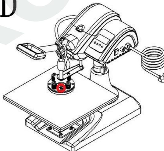
Remove the heat platen and install the plate heater
