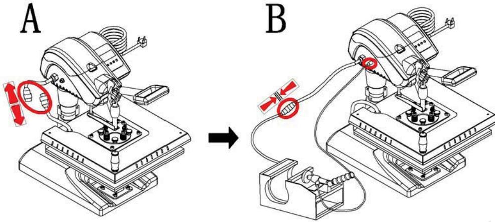
Disconnect the heat platen wire. Connect the mug press, one socket is power socket, the other one is limit switch socket.
