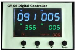
Press button to operating mode. Counter is "transfer cycle", from 0~999.Press "Reset" for 5 seconds to make the counter to be "0".
