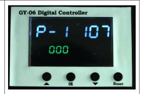
When the temperature shows on the display is not the same as actual temperature on heat platen, press button for 5 seconds to reset mode:
