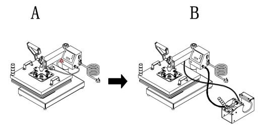
Disconnect the power connector of heat platen as the above picture shown.
