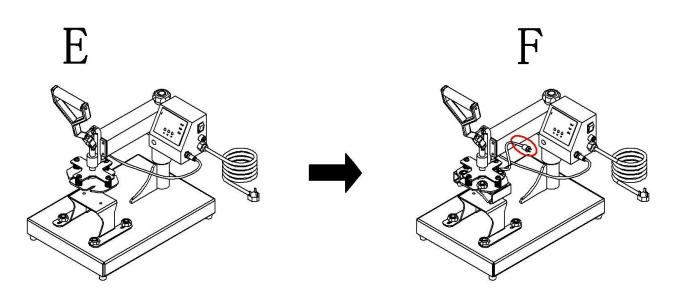
Tighten the screws of cap heat element, then connect the wire to the power connector.
