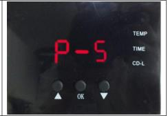
If there is a difference between the actual temperature and temperature shows on the controller, you can use **P5 mode** to calibrate the difference.
