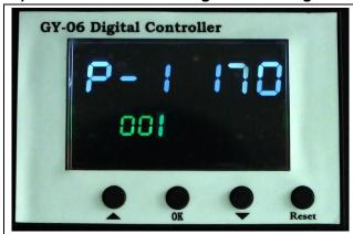
When there is temperature difference between SV (current heating temperature shows on the display screen) and actual Temp of heat platen, please long press button for 5 seconds to enter the P-1 mode to calibrate.
